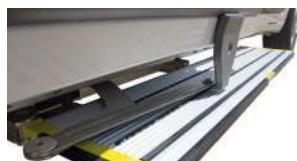
Minimal door stroke for full step deployment.
